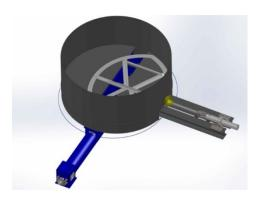
A silo with sliding frame is a silo with, for extraction system, a sliding frame. The bottom of the silo consists of a moving frame that will convey the product to an extraction screw.
