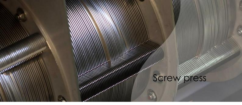
The Disc Screw Press is a screw press for dewatering of sludge and solid waste. The sludge is conveyed by a screw through a tube composed of rings / discs. By rotating the screw, the discs move and the filtrates are drained by / between the discs.
